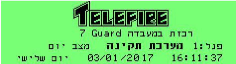
Figure 1: Normal operating mode (the line below the manufacturer logo can be changed)
